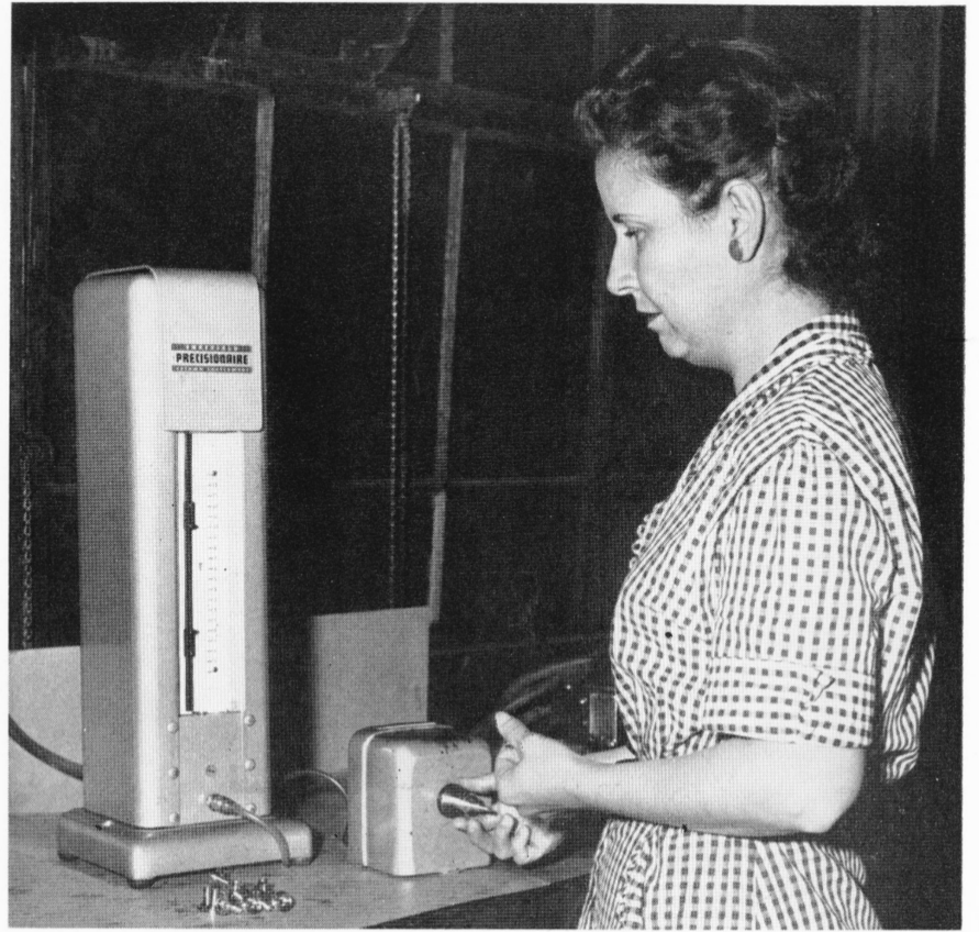
Eunice Barrows of ASMD is inspecting a piece of work for tolerance on the recently-purchased Sheffield Precisionaire. She finds it easy to read because of its extremely legible scale and highly visible pointer.
